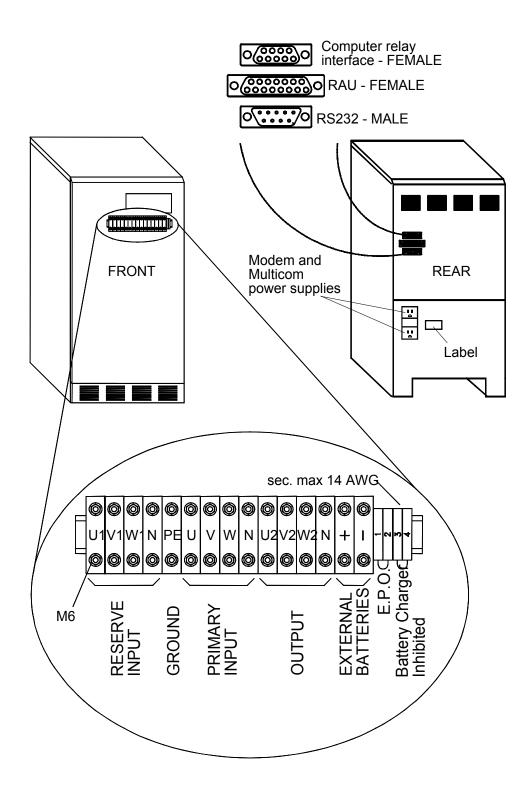
Figure 20 - 24 – 12/18/24kVA: Cable Connections
